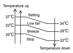
• In heating operation, if air conditioner turn off, the indoor fan motor will run most for 30
