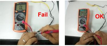
3) The PCB fail. Solution: Replace the indoor main PCB.
