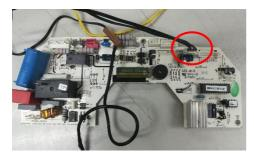
2) Room temperature sensor (IRT) and Indoor pipe (coil) temperature sensor (IPT) damage (short or broken).
