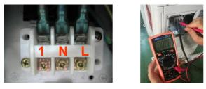
5) Communication fault if resistance or optical coupler broken, replace outdoor PCB.
