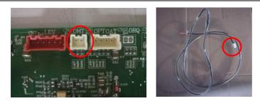
**Solution:** Check the connecter of sensor and slot, if loose or not plugged in, please connect again. 2) Outdoor pipe temp sensor damage.
